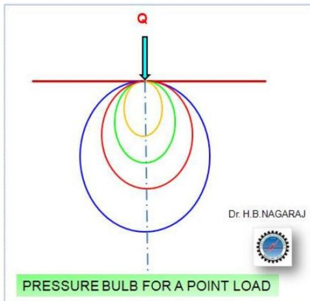
**Fig. 3.3 Pressure bulb for a point load**
